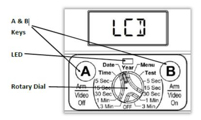
Rotary Dial is used to access camera settings, arm the camera, and to turn the camera off.
