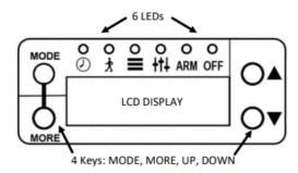
Set the Date - Press the More button after setting time to move to the date. Press the Up arrow to get to the month. Use the Up/Down arrows to change the month. Press the More button to move to the day. Use the Up/Down arrows to change the day. Press the More button to move to the year. Use the Up/Down Arrows to change the year.
