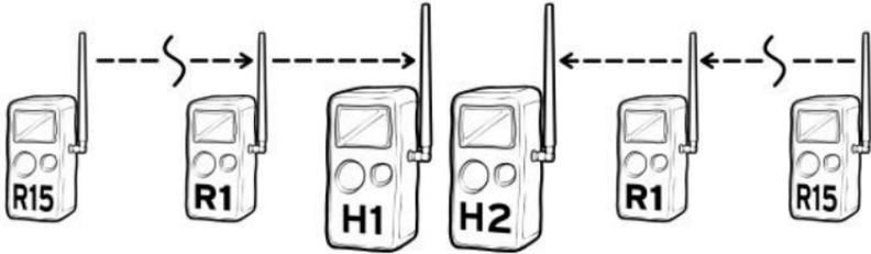
*If you require more than 24 remote cameras you can deploy two networks on different channels. The Home cameras can be near each other.*
