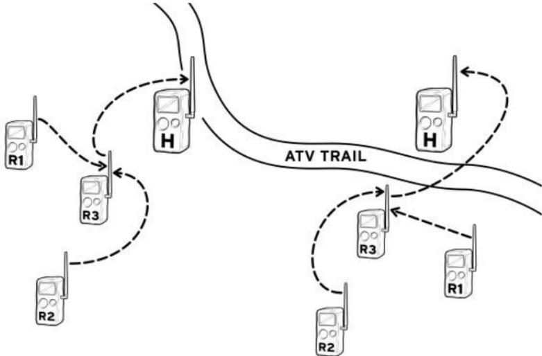
*On large properties you can deploy multiple networks in various locations. For example, instead of linking distant cameras create multiple networks.*
