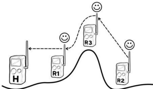
*Use a repeater to extend range. A repeater is the best way to transmit over a hill or ridge.*
