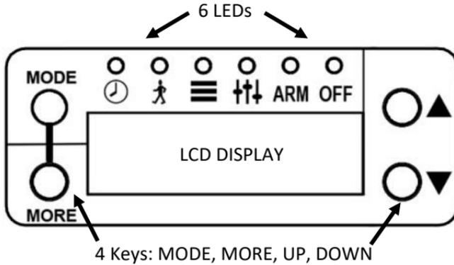
Press the **MODE** key to change the operating mode. The corresponding LED will light to show what mode is enabled.
