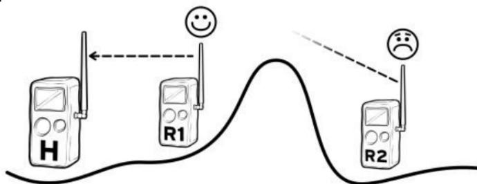
*A hill can block the radio signal*
